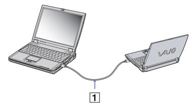
If the notebook is connected to the optional docking station, proceed as follows to exchange data with another computer using an i.LINK™ cable (optional):
